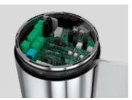
BOARD Featuring a display that is built-in to the automation, enabling fast, easy function control.
